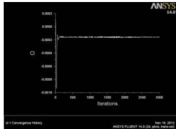
Figure 12: Graph of coefficient of Lift at zero degree of AOA.
