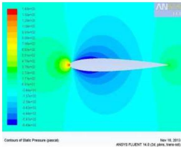
Figure 5: Contours of static pressure over NACA 0012 airfoil at 0 degree of AOA
