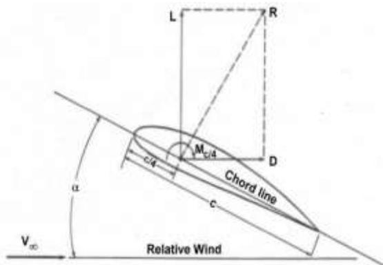
Figure 2: Angle of attack
