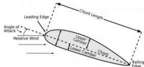
**Figure 1: Basic nomenclature of an airfoil**
